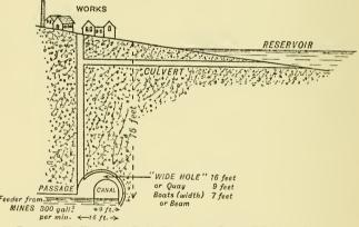
FIG. 25.-SECTION OF TUNNEL. "WIDE HOLE" AND QUAY.
